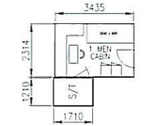
DETAIL 3 TYPICAL 1 MEN CABIN ARRANGEMENT SCALE 1:50
